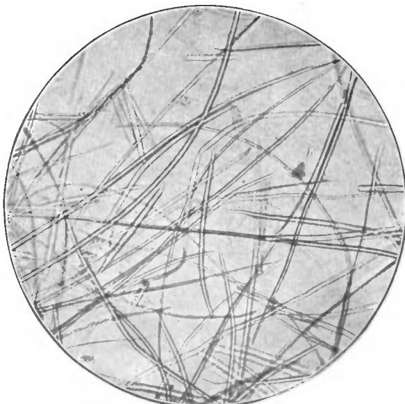
FIG. 11.—ESPARTO. Cellulose. Ultimate fibres of paper making pulp. Typical fusiform bast fibres, with scattered serrated cells of cortex and hairs. \times 65 .
