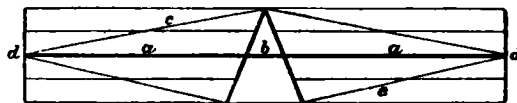
FIG. 42.—Wenham's system of Aeroplanes designed to carry a man. a, a, Thin planks, tapering at each end, and attached to a triangle. b, Similar plank for supporting the aeronaut. c, c, Thin bands of iron with truss planks a, a, and d, d, Vertical rods. Between these are stretched five bands of holland 15 in. broad and 16 ft. long, the total length of the web being 80 ft. This apparatus when caught by a gust of wind, actually lifted the aeronaut.
