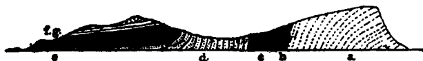
FIG. 1.—Section of the Isle of Wight—a Monoclinial Curve. a , Chalk; b , Woolwich and Reading beds; c , London clay; d , Bagshot series; e , Headon series; f , g , Osborne and Bembridge series.
