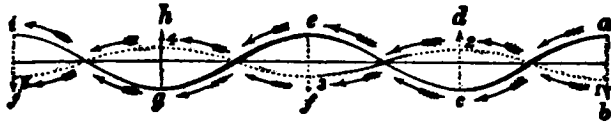
FIG. 29 shows how in progressive flight the wing and the body describe waved tracks ,—the crests of the waves made by the wing ( a, c, e, g, i ) being placed opposite the crests of the waves made by the body 1, 2, 3, 4, 5 .
