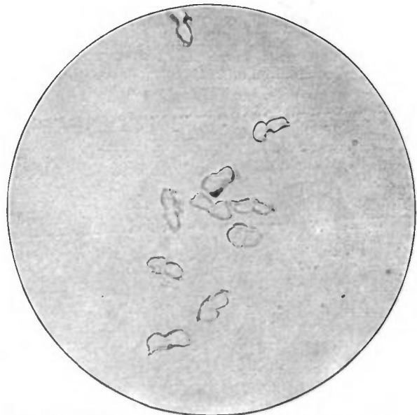
FIG. 2.—RAW SILK. Bombyx mori . Single fibres in transverse section showing each fibre or "bave" as dual cylinder. \times 235 .
